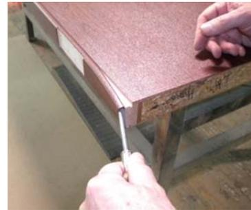
Step 2: From this point, slide the screwdriver down the length of the door on the wide face, releasing the return leg over the entire door length. Detach the vinyl from the door by lifting it from the return groove on the narrow face.
