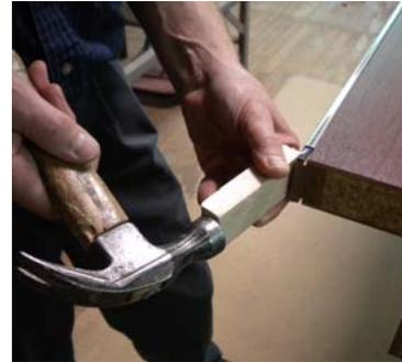
Step 2: A strip of tape should remain attached to the edge of the door on both the wide and narrow faces. This tape insures proper fit and aids in the impact resistance of the edge and should not be removed.
