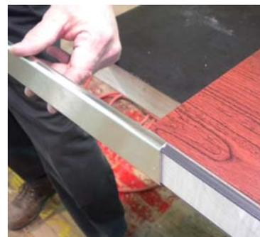
Step 4: Continue sliding the edge onto the door until it is properly aligned with the ends of the door. Reattach any hardware removed in step 1.
