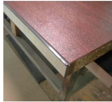
Step 3: Begin attachment of the replacement edge by compressing the tape at one end of the door and sliding the replacement edge over it.
